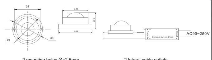
2 mounting holes Ø=2,5mm, distance: 34mm
